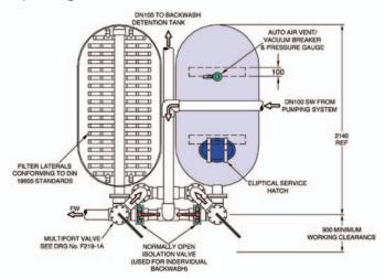
Tandem filter systems are a compact and efficient means of providing effective filtration for all sorts of small commercial pools. With features such as compact size, low pressure drop, and easy maintenance, it's no wonder that **MHS 1500** and **MHS 1800 G2** filters are acclaimed by contractors and owners alike.
