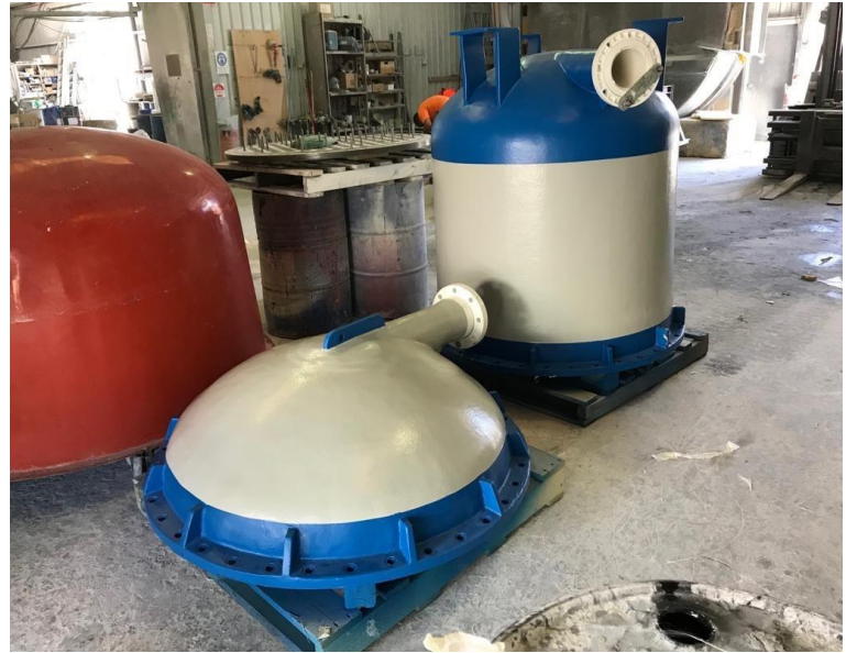
Barrel and dished head – Subassembly,
