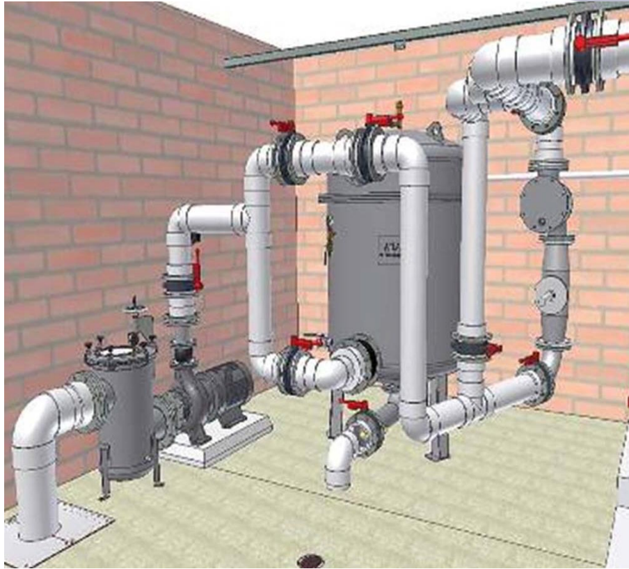
Typical installation schematic with U/V sterilization
